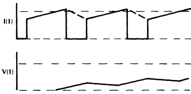
Figure 4. Switching Current and Pin 4 Voltage — Normal
